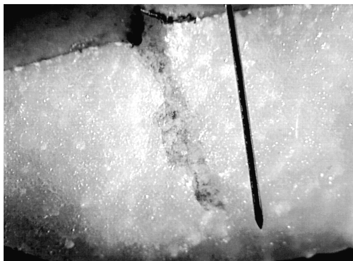
FIG. 2—Cross section of puncture in pear. A control needle is pictured next to cross section of hole. Oxidation has taken place in the hole so the needle bore is more visible.
